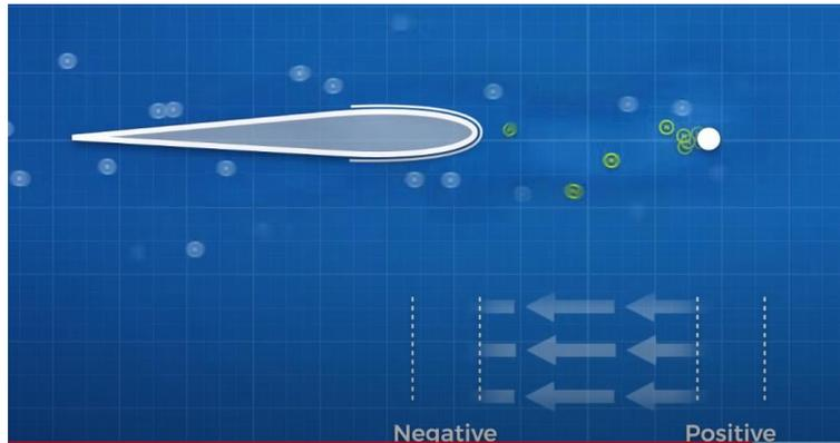
Figure 1 Ionic wind | Note the flow of charged atoms from the positive to negative end and the subsequent interaction with neutral atmospheric particles. Also, note the shape of the foam glider, maximising lift provided. | Courtesy: Real Engineering
