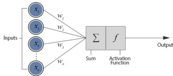
**Neural Networks are inspired by the human brain** - this perceptron configuration takes a number of weighted inputs and "fires" if the sum is greater than a certain value via the activation function, similar to how synapses fire if the excitatory input is larger than the inhibitory input. The output is compared to the training data and the weights adjusted until the system "learns". (Reproduced from [6])
